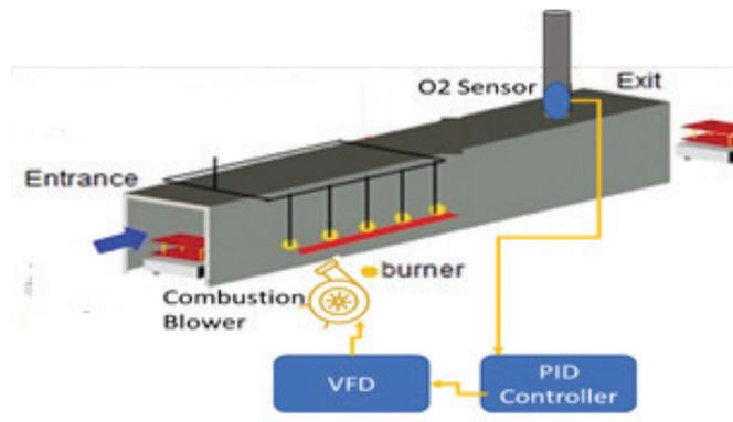
Figure 73: PID & VFD based excess air control system
