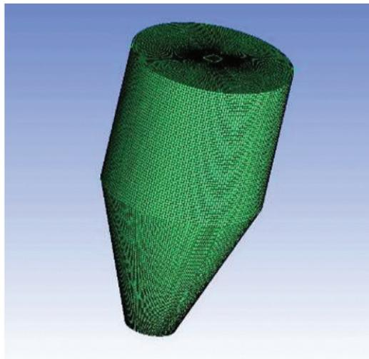
Figure 57: CFD Model of main drying chamber
