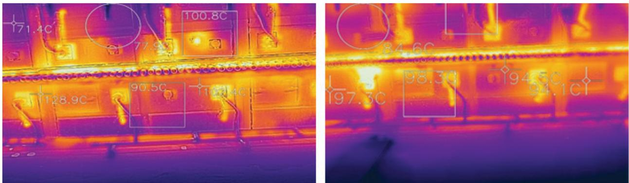
Figure 31: Thermal Image of Roller Kiln
