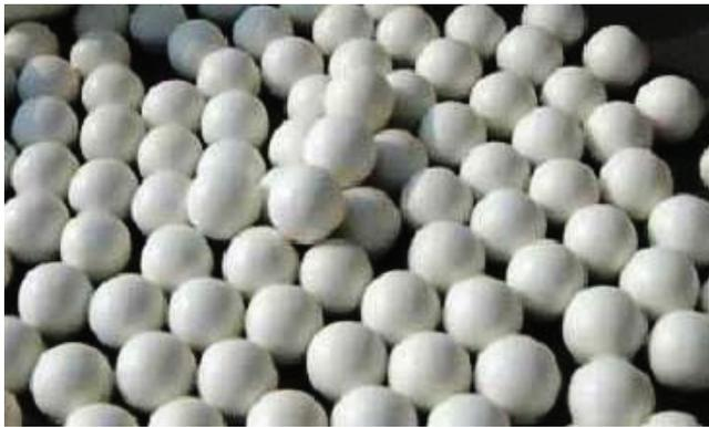
Figure 77: High alumina balls
