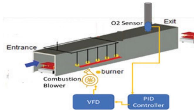
Figure 33: PID & VFD based excess air control system
