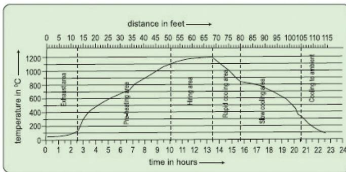
Figure 70: Firing Cycle
