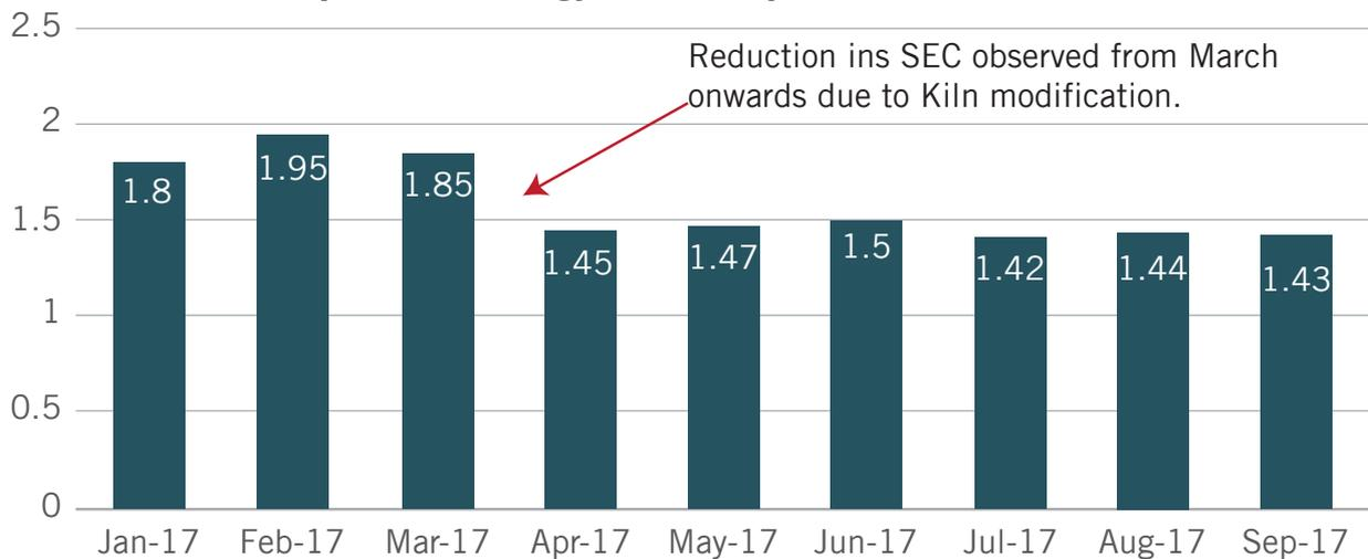
Figure 27: Reduction in SEC after implementation of WHR system
