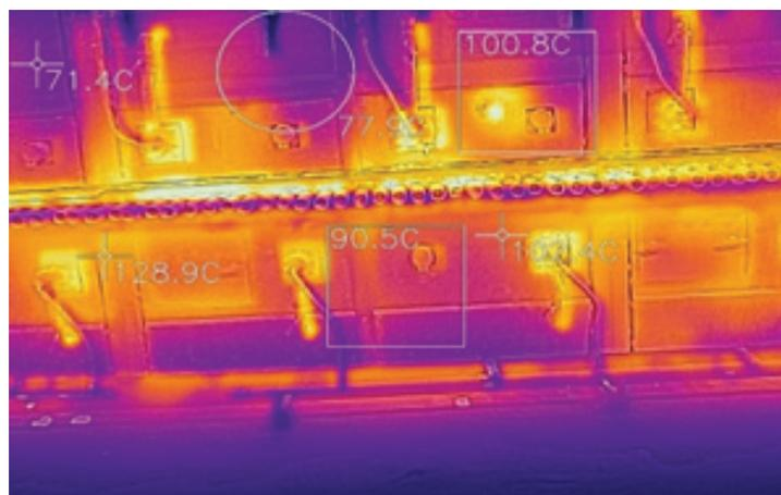
Figure 29: Surface temperature at firing zone in roller kiln
