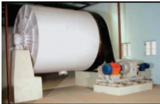
Figure 34: Conventional Ball Mill system
