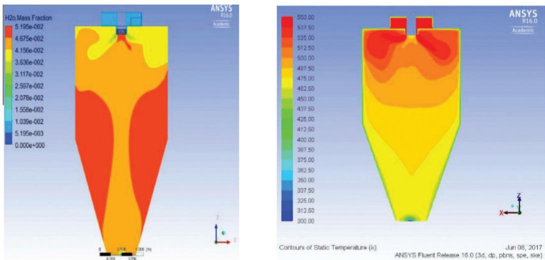
Figure 58: Contours of moisture concentration and temperature distribution inside the chamber
