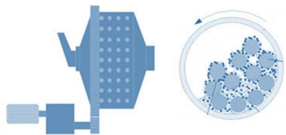
Figure 4: Raw material blending (wet ball milling)
