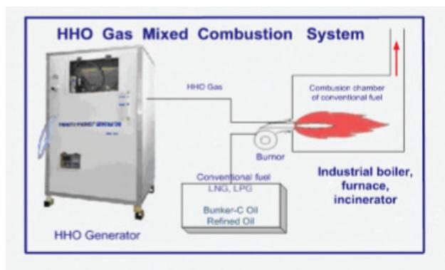
The ceramic unit can have hydroxy mixed combustion system (min 5% of total energy) to mix with natural gas in kiln firing and burn Hydroxy Gas with conventional fuel to achieve fuel savings. Hydroxy Gas Generator unit supplies Hydroxy Gas 24 hours into the combustion chamber of existing facility. The Hydroxy Gas is mixed with conventional fuel and burned together. This can result in saving of 5-10% in fuel consumption.
