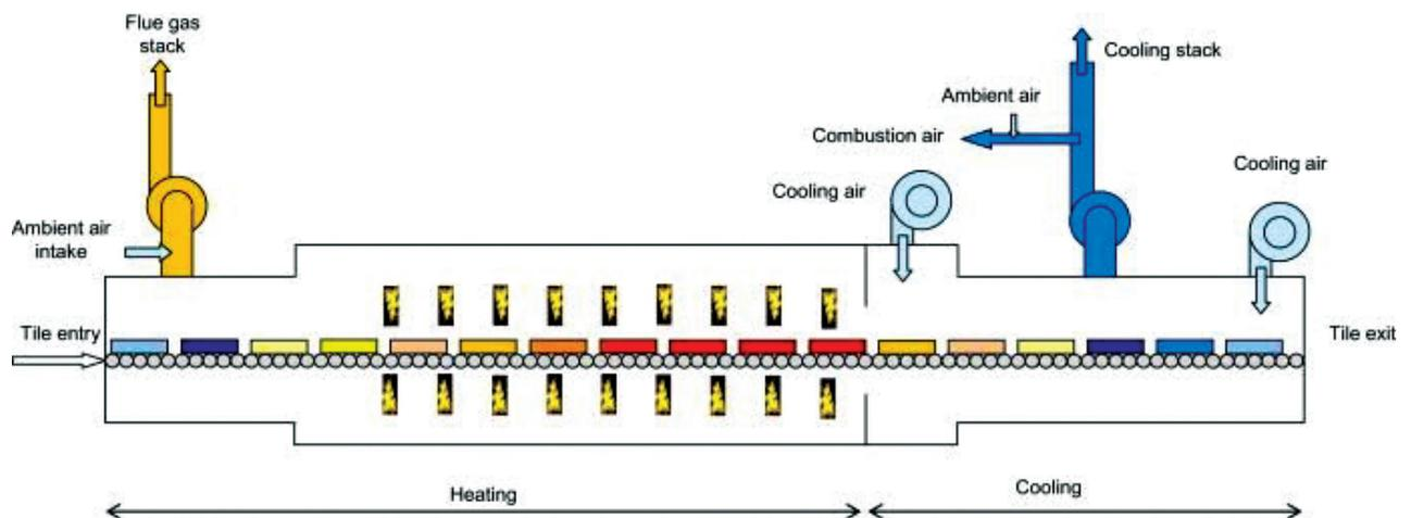
Figure 10: Tunnel Kiln firing
