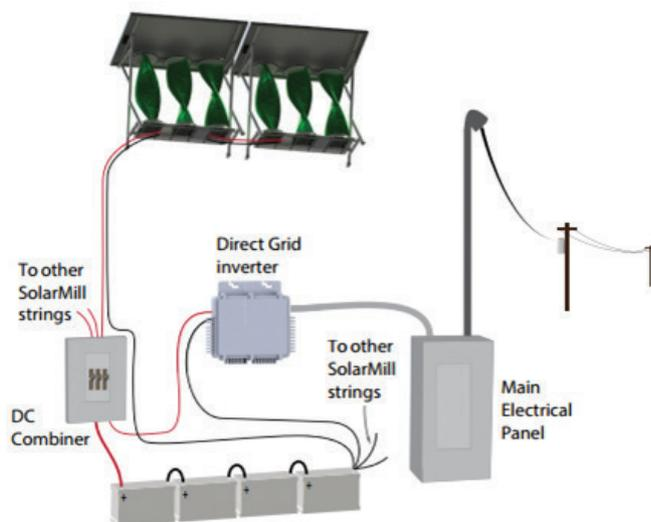
Figure 84: Hybrid mill connected to supply
