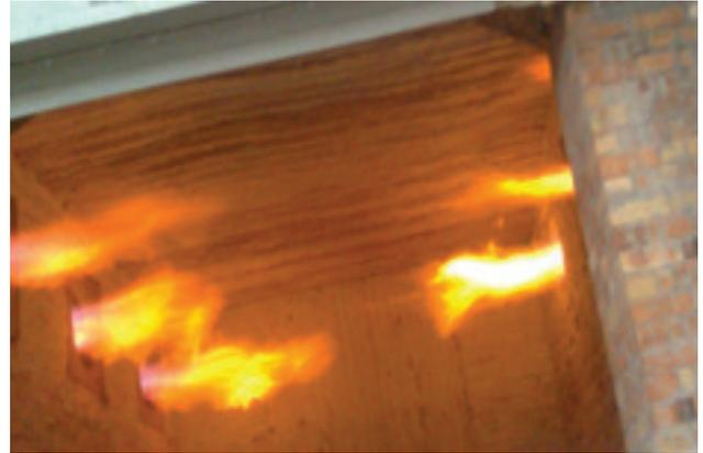
Figure 90: Improper air to fuel ratio
