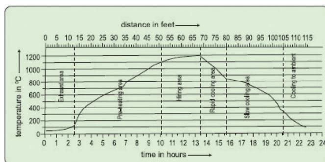
Figure 19: Firing cycle
