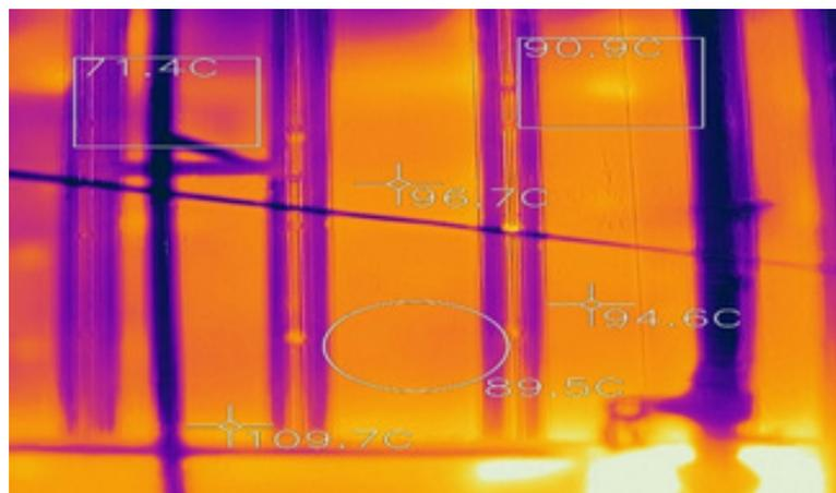
Figure 67: Surface temperature at firing zone in kiln
