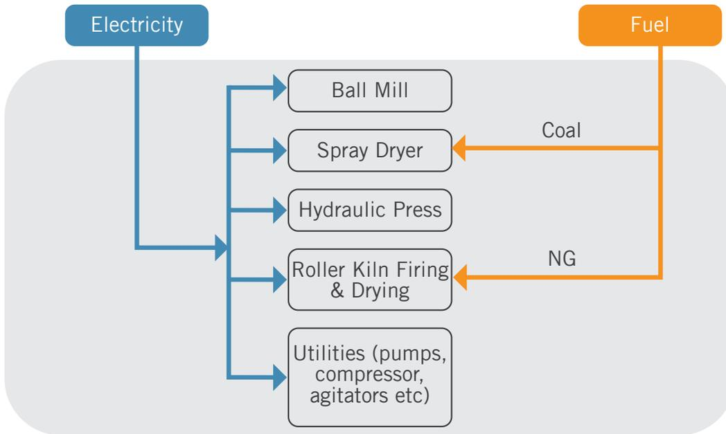
Figure 23: Ceramic tile manufacturing unit – Energy usage area
