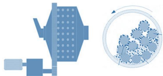
Figure 13: Raw material blending (wet ball milling)
