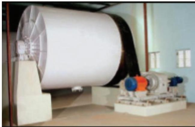
Figure 74: Conventional Ball Mill system
