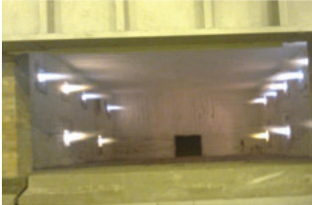
Figure 89: Perfect combustion with correct air fuel to ratio
