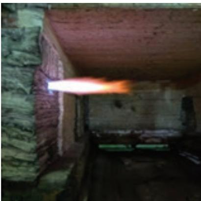
Figure 88: High Velocity Burner with Flame
