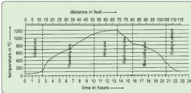
Figure 11: Firing cycle
