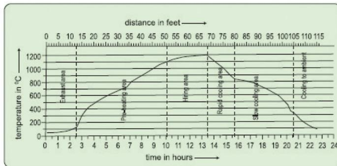
Figure 30: Firing Cycle
